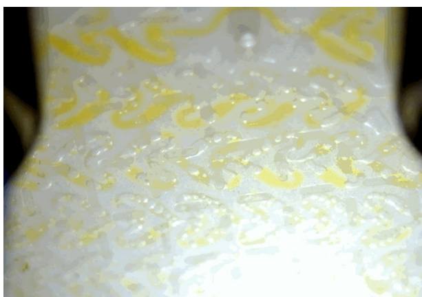
Figure 4: Gas-liquid reaction under continuous-flow conditions in a mesofluidic device showing details of heart-shaped static mixers (Courtesy of Corning®)
